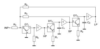
Figure 1: Multifunctional KHN filter using DT-s and buffers in VM.
