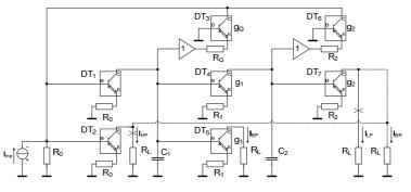
Figure 5: KHN filter using DT-s and buffers in CM
